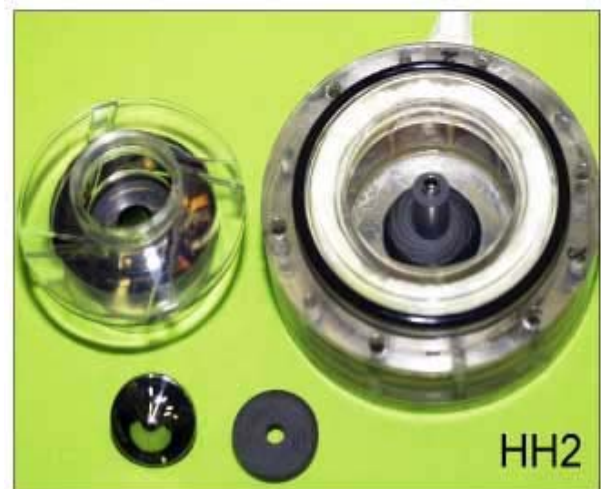
Hydrodynamic levitating centrifugal pump
