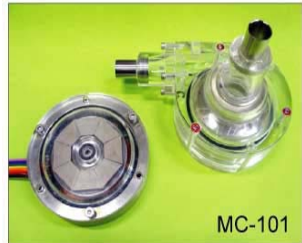
Monopivot centrifugal pump
