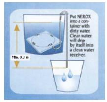
the membrane can be cleaned and re-used over and over. A single filter can process up to 2.500 liters.
